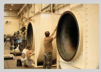
Stainless Steel Inlet Filters FanAir designs and builds many types and styles of Filter Banks in Stainless Steel, Mild Steel and Fiberglass, using Stainless Mesh Filters, Polypro Filters, Pleated Filters and HEPA Filters.
