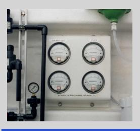
Dwyer Instruments 2000 Series Magnehelic Gages mounted and plumbed are standard on all Grease Filters and Mist Eliminators.
