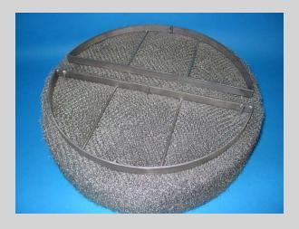
Mesh Pad Type Thermoplastic and Stainless wire mist eliminators, or knitted mesh pad mist eliminators, collect droplets by the inertial impaction and interception mechanisms of collection. Mesh Pad separators are commonly used to collect droplets above 5 microns in diameter.
