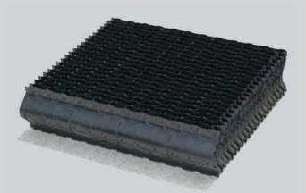
Chevron type impaction Mist Eliminator profiles are available in both Horizontal and Vertical blade configurations. Saturated air moving across the blade section impacts the stacked vanes and is drained to the low pint of the mist eliminator housing.
