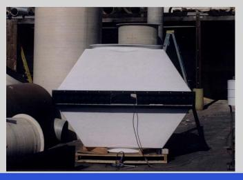
FanAir Company Can furnish either horizontal or vertically mounted with options for single and two stage filtration. Chevron type mist eliminator blades Mesh Pad section are available to remove moisture before or after wet chemical process equipment.
