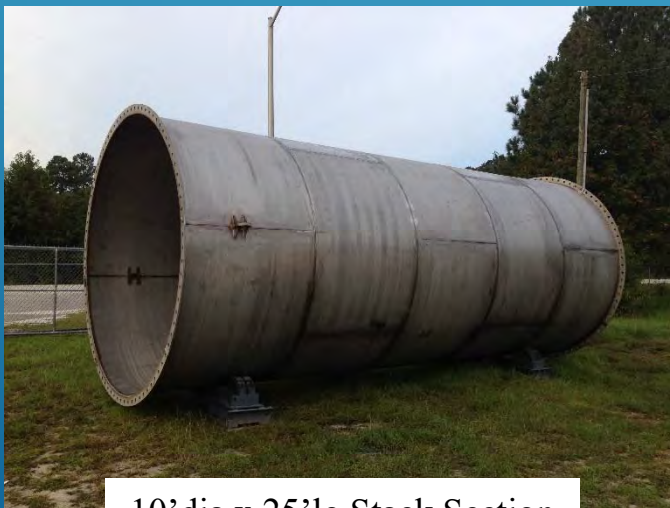
10'dia x 25'lg Stack Section
