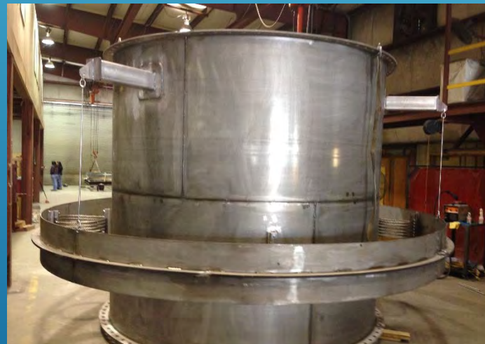
10'dia x 10'lg Top Stack Mass Tune Damper
